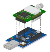
To install an mDot on the Micro Developer Board:
