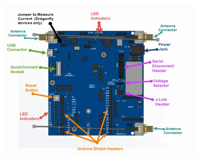
**Note:** The development board derives power from the USB connection. The Power Jack connects to the Arduino shield socket. If the Arduino shield needs 5 V, use a 5 V power supply. A 9 V supply will not be regulated down to 5 V.
