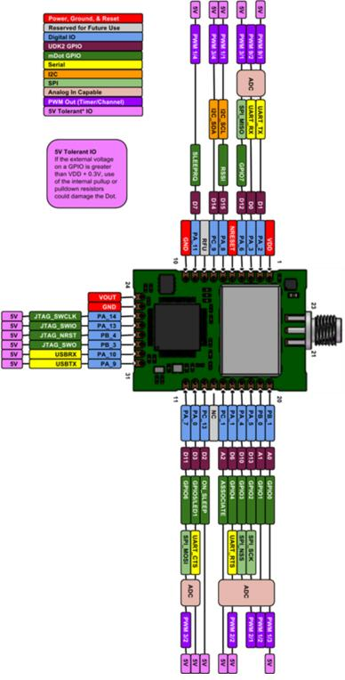
Note: Using the mbed platform with the Cortex-M4 processor expands your pin functionality options.
