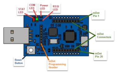
Note: The Reset Button resets the mDot processor.
