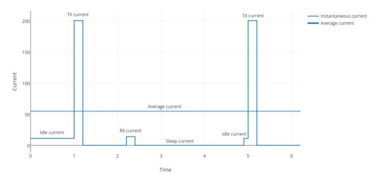
Use the current consumption values from the following Electrical Characteristics table when calculating average power consumption.
