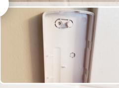
Use the included large adhesive pad to secure the case to the wall. For increased security (optional), fasten the case to the wall using the included tamper screw as shown.
