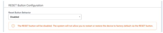
**NOTE:** Disabling factory default settings means there is no mechanism to restore the device to commissioning mode. Do not lose track of your login credentials or you will lose access to the device.
