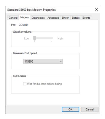
In **Device Manager**, open **Ports (COM & LPT)** and then right-click on the Com Port used by your device and select **Properties.**
