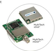
The mDot and xDot are LoRaWAN compliant,
