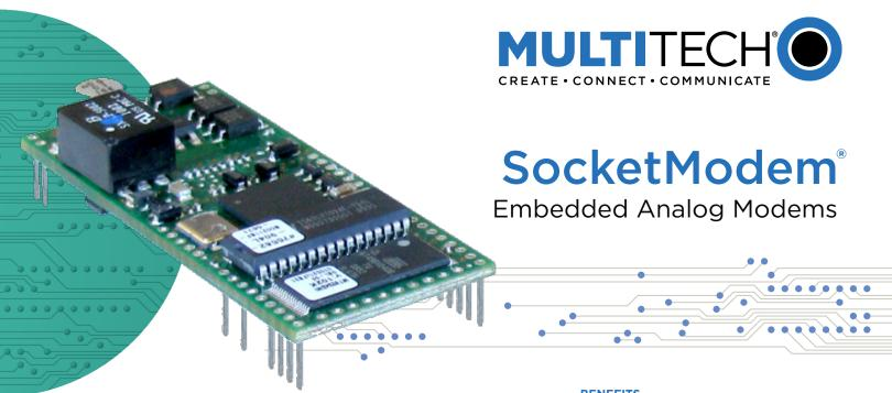
MultiTech SocketModem\* embedded modem creates communication-ready devices by integrating data/fax modem functionality into a single, universal socket design. It utilizes a space-efficient (1" x 2.5"), design that allows OEMs to integrate a wide range of modem functions and speeds into any product platform. The SocketModem embedded modem complies with telecom requirements globally and can be shipped worldwide.
