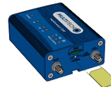
If you want to operate the modem on a particular cellular network, install a mini-SIM card (2FF form factor).
